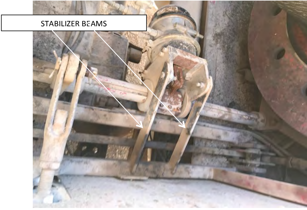
1.8 Weld Stabilizer Option 2: Weld stabilizer (not supplied by PTS) on the top brake harness plate and connect to Stabilizer Clevis (not supplied by PTS)
