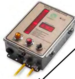
When the limits are reached the Posi-Stop console will send an electrical current to the Solenoid Valve which will cause the valves actuator to close the air port to the clutch and throttle and open the port to send air to the service brake side of the brake canister. Once air is sent to the brake the brake's piston will extend and engage the band brake
